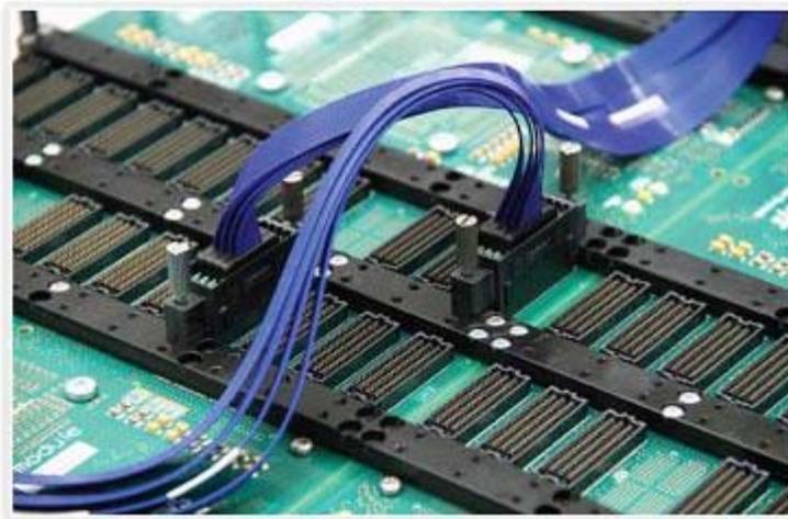
[ Figure 3: Enhanced HapsTrak 3 connector technology supports high-speed I/O interfaces ]
