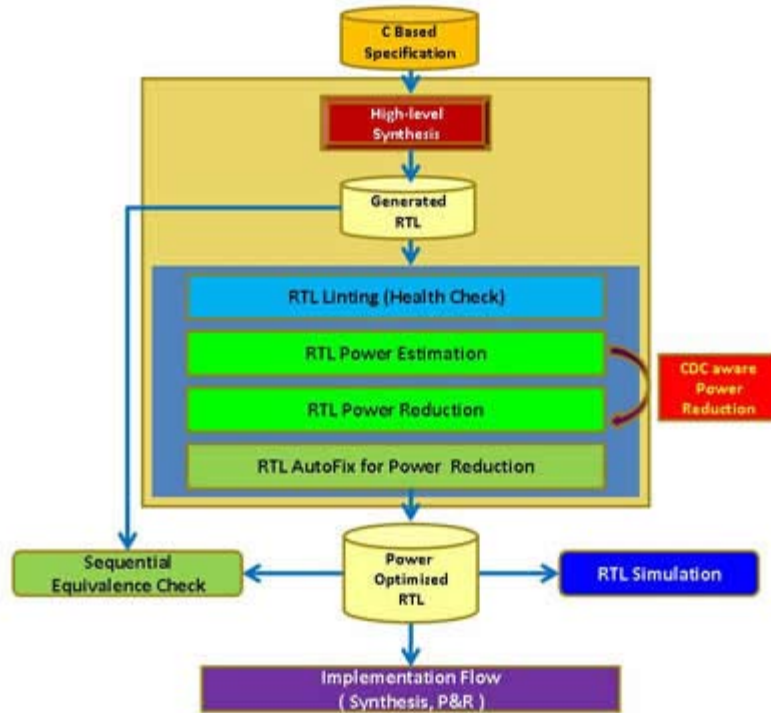
[ Figure 2: Integrated high-level synthesis & power optimization flow ]
